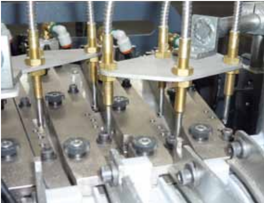
Sensors monitor and regulate the feeding of the nuts into the feeding lines.
