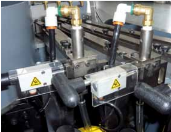
One stud at a time is blown from the sensor-monitored shuttle into the tool and is installed subsequently.
