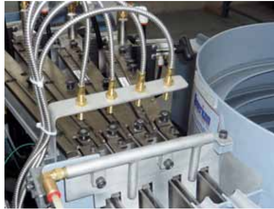
Sensors monitor and regulate the feeding of the studs into the feeding lines.
