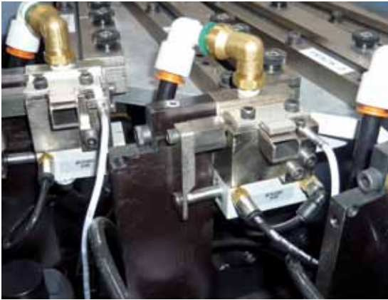
One nut at a time is blown from the sensor-monitored shuttle into the tool and is installed subsequently.
