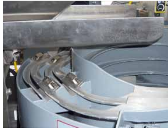
The nuts are pre-sorted in an escapement into the correct direction for installation.
