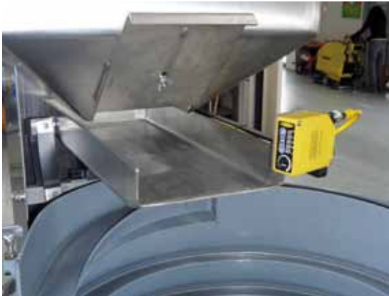
The bunker, also sensor-controlled, guarantees a constant filling level of the bowl.
